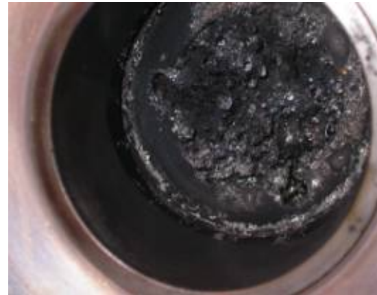
(b) Exit of Uncoated 35Cr-45Ni-Fe Reactor (no S – ethane run)
